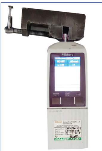
[Table/Fig-3]: Surface roughness testing in Surface Profilometer. [Table/Fig-4]: Flexural strength testing in universal testing machine.
